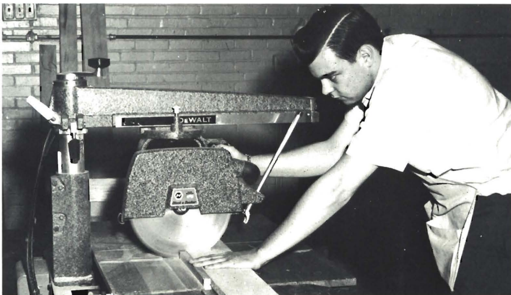
The Radial saw is one of the new pieces of machinery being used in the machine shop.
