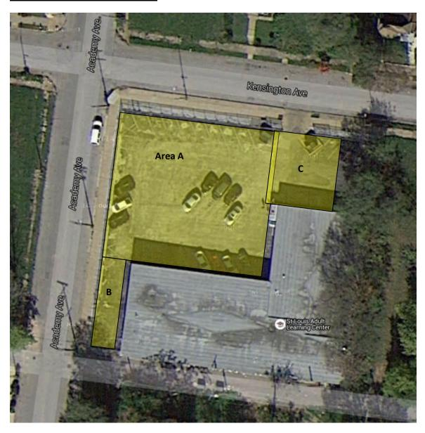
• Excavate rock base, re-rock, pave with 2-1/2" of asphalt, and restripe parking lot in Areas A, B, and C.
