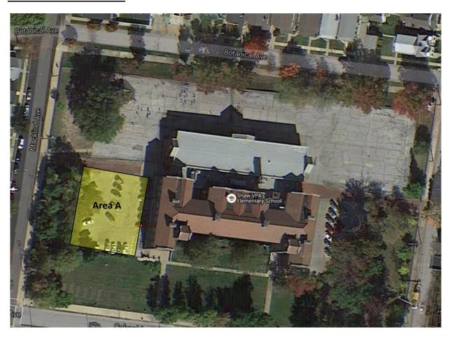
• Excavate rock base, re-rock, pave with 2-1/2" of asphalt, and restripe parking lot in Areas A.
