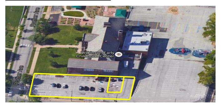
• Excavate rock base, re-rock, pave with 2-1/2" of asphalt, restripe parking lot, and install concreate pad within yellow boarders.
