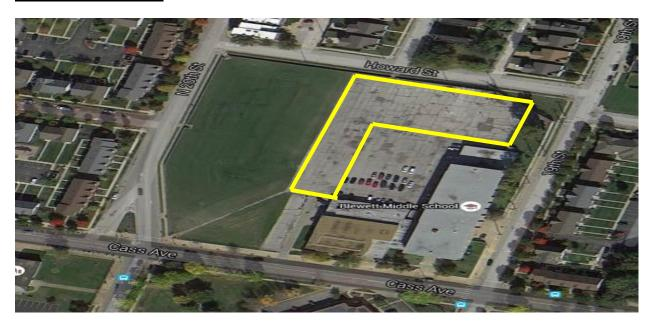
• Excavate rock base, re-rock, pave with 2-1/2" of asphalt, and restripe parking lot within yellow boarders.
